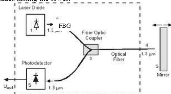
Fig. 6: Fibre optic displacement sensor schematic [2]
