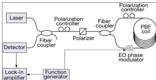
Fig. 5: Fibre optic Gyroscope[2],[11]
