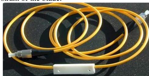
Fig. 3: Fibre Bragg Grating module[11]
