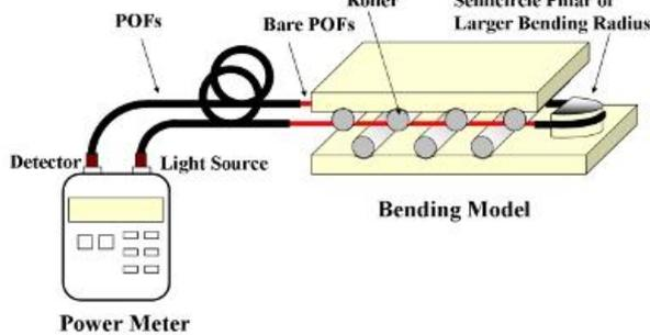
Fig. 4: Fibre optic Microbending Sensor [2][11]
