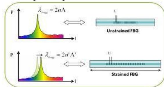
Fig.2 : Fibre Bragg Grating principle[11]
